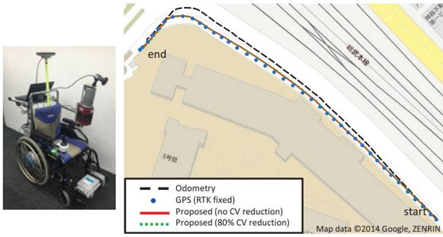
Fig. 8. Left: robot used to collect data. It is equipped with a Point Grey Flea3 camera, a Velodyne HDL-32e laser scanner, a gyro and a GPS receiver (Ladybug was not used). Right: result of position tracking experiments. The red trajectory shows the result of our method without reduction of cross-validation procedures. The green trajectory shows the result with 80% of cross-validation reduction.
