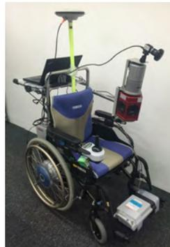
Figure 9. Robot used to collect datasets for position tracking experiments. It is equipped with a 3D LiDAR, an omnidirectional camera, a monocular camera, a gyro and a GPS receiver.
