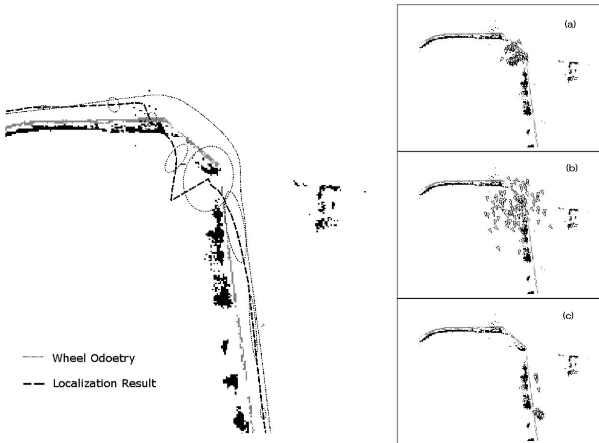
Figure 15: Recovery from localization failure. Left: estimated position and error ellipses. The trajectory obtained by gyro-assisted wheel odometry is shown for comparison. The robot navigated from top- left to bottom- right in this figure. Right: distribution of particles. The triangles show particles. The red triangles show estimated position. (a) Localization is incorrect due to visual odometry failure. (b) Kidnapping is detected. (c) Robot re-localized.
