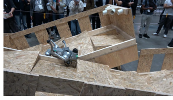
Figure 9. Failure to get up after falling
