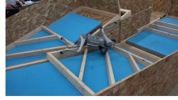
Figure 10. Failure of self-localization after falling
