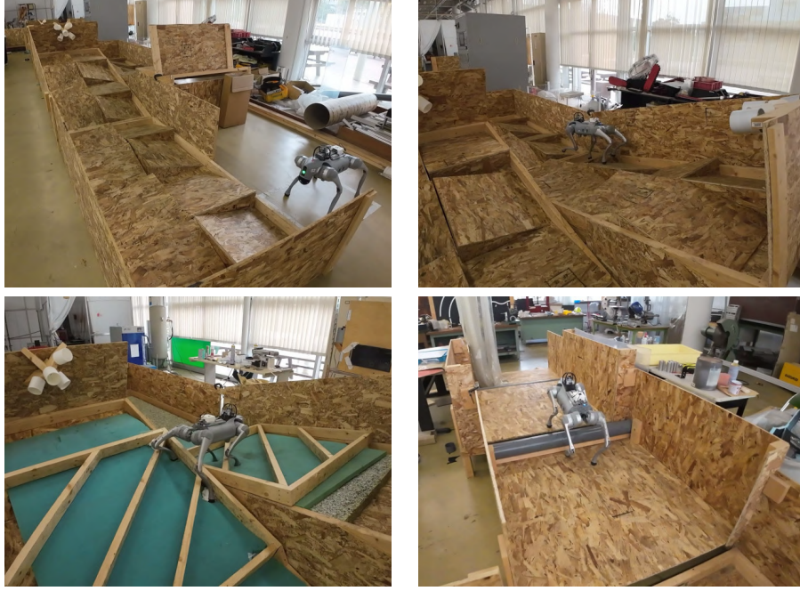
Figure 11. Experimental setup for escape strategy comparison
