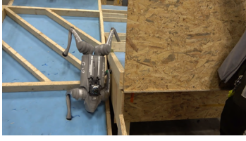
Figure 8. Failure because of abnormal state of the lower layer after being stuck
